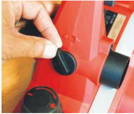
▲ The side from which the shavings eject is controlled via this small dial
